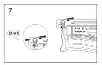
7. Once the butt pad is removed you must lower the feed ramp before attempting to remove the
