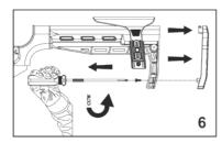
**6.** To remove the upper receiver from the lower receiver, you must start by removing the butt pad screw to gain
