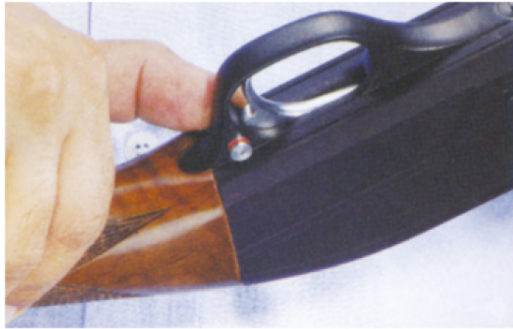
In the "off safe" position, a red warning band is visible on the safety button on the left side of the trigger guard. The gun can fire. (Photo 1)
